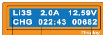
number of cells    charging time    charge current    battery voltage    charged capacity
